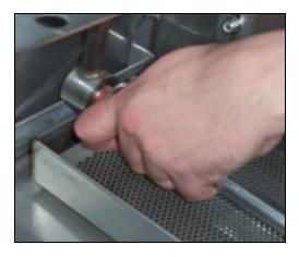
Unscrewing and removing the lower rinse arm
